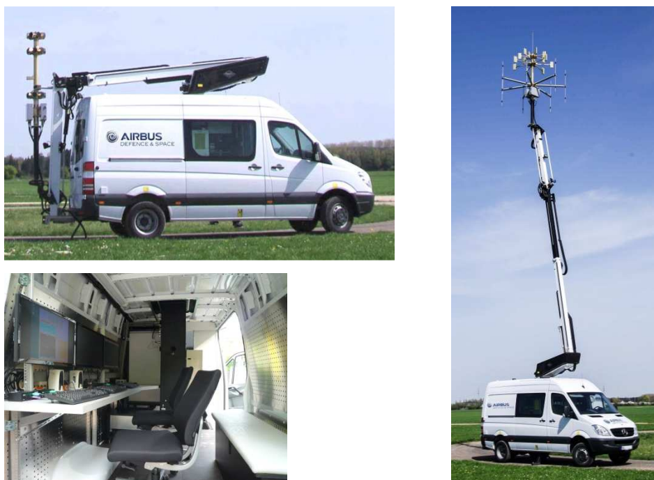
Figure 2: Passive Radar van and operator consoles (Courtesy of Hensoldt).
